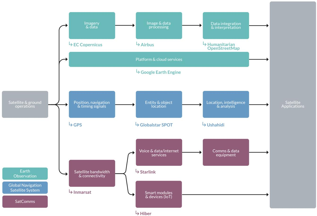
FIGURE 12: Components of Satellite Applications
